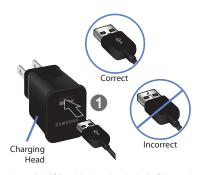
2. Insert the USB cable into the device's Charger/ Accessory Port (2).
